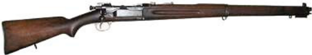
Krag-Jørgensen 1889 7.87mm (0.31) or 7.62mm (.30-40 Krag) or 6.5mm Nor (0.256 in) 5 rounds Bolt action
