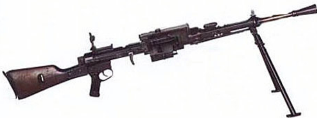
Breda M30 1930 6.5mm 20 rounds 450-500 rpm Note: Has folding bipod
