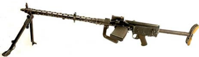
MG13 1932 7.92mm Mauser 25 or 75 rounds 550 rpm Note: Has folding bipod
