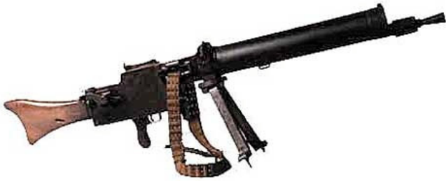
MG08/15 1915 7.92mm Mauser 250 round belt 300-450 rpm Note: Has folding bipod
