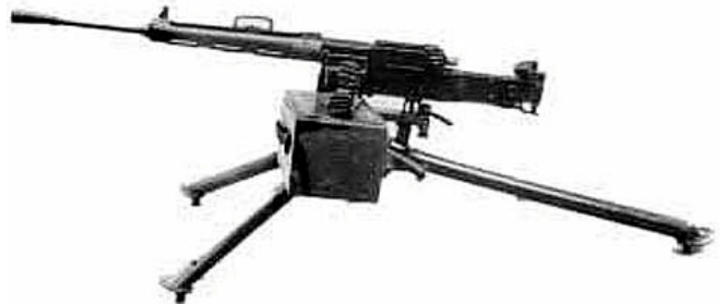
Fiat Revelli M35 1935 8mm Breda 50 round belts 500 rpm Note: Tripod or vehicle mounted
