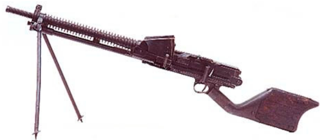
Nambu Type 11 1922 6.5mm 30 rounds 500 rpm Note: Has folding bipod
